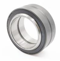
For bearings operating at high permanent loads or in the one-sided load direction, the rings are provided with grooves and holes for periodic re-lubrication. For this purpose, use normal running greases, preferably with the addition of molybdenum disulfide or lithium greases.
